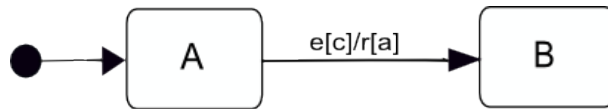
Figure 1: Two basic states connected by a transition originating from the initial state on the left.
