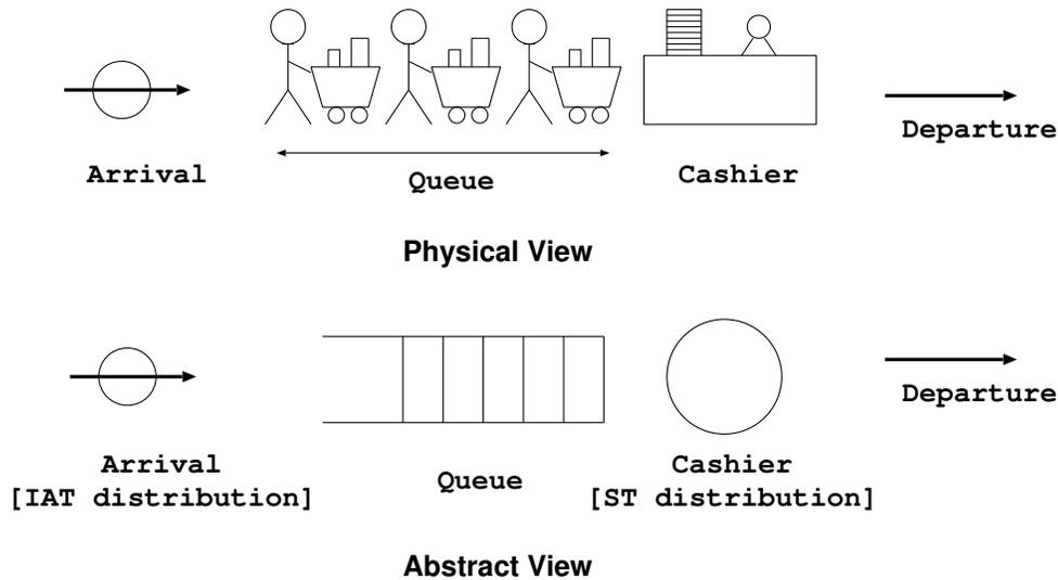
Figure 7: Simple single queue, single server system
