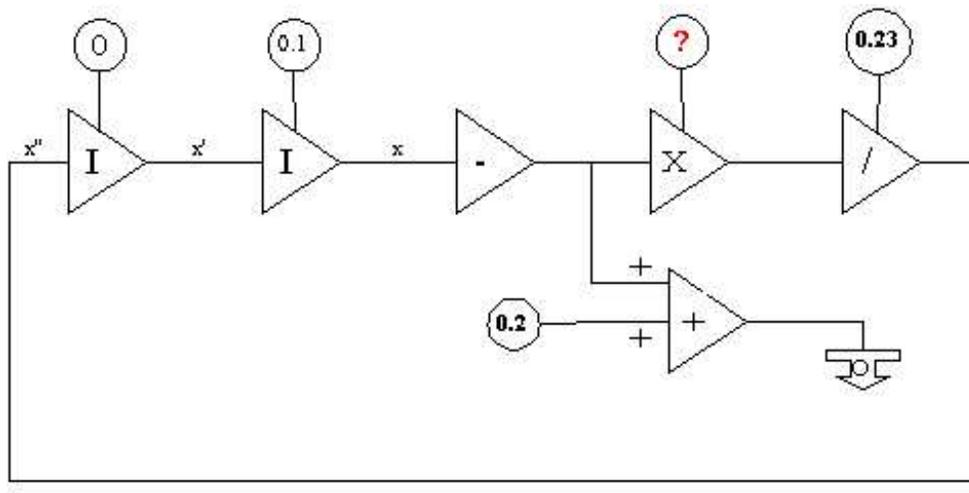
Figure 12: A causal block diagram model for the Mass-Spring problem
