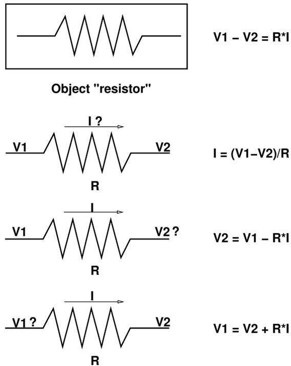
Figure 13: Electrical resistor
