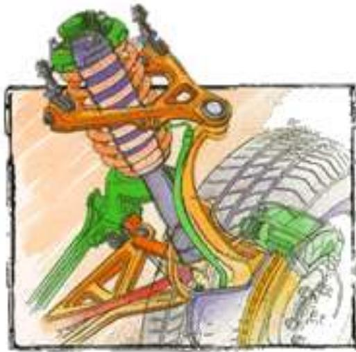
Figure 16: Car suspension, physical view
