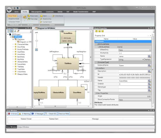
Figure 1: Creating the RPG metamodel in VMTS
