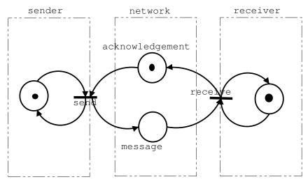
The above Petri Net models a simple communication between a sender and a receiver. It is assumed messages are not lost nor damaged. A token in the sender place means the sender is ready to send. A token in the receiver place means the receiver is ready to receive. A token in the acknowledgement place means there is an acknowledgement (of receipt) message on the network. A token in the message place means there is a data message on the network.
