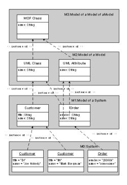
Figure5. An example in MOF meta-model framework
