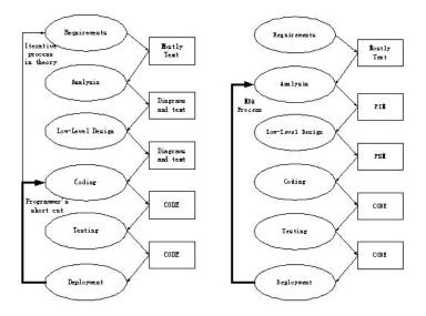
Figure 1. Traditional software development process Figure 2. MDA development process Although they both consist of the same six stages in their life-cycles, there're several distinguished features in a MDA process
