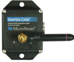
Figure 4.1. MicroStrain Inertia-Link ® IMU.
