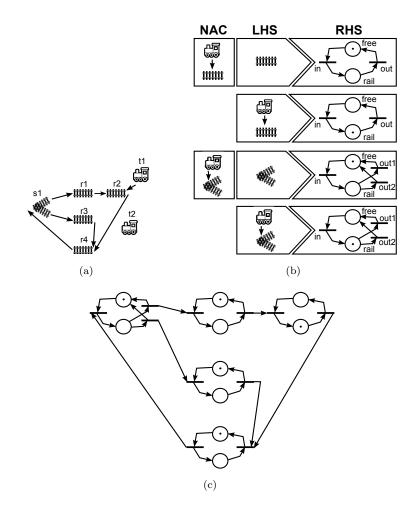
FIGURE 3.2: (a) An example TrainSim model, (b) The TrainSim-to-PetriNet transformation (semantic mapping), in the form of rules, (c) The resulting PetriNet model.
