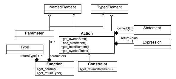
FIGURE B.6: The ArkM3 Action and Constraint metamodel.
