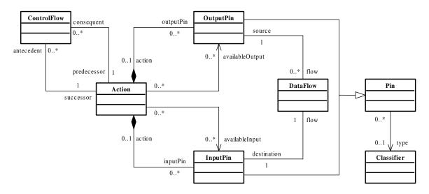
Figure 4: The minimal core of the action semantics package
