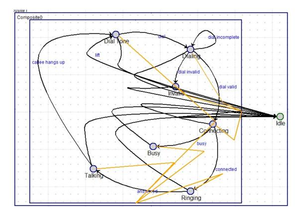
In order to finish the experiment successfully there is only one refactoring to be done. That is the fold outgoing transitions rule which should fold all those incoming transitions to the state Idle into one transitions going from the Composite0 to Idle.
