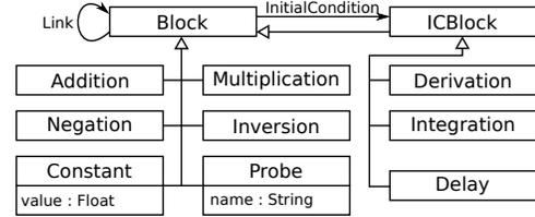
Figure 1. Causal Block Diagrams metamodel.
